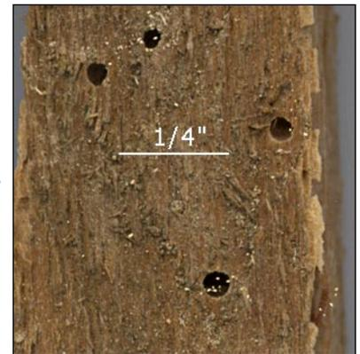
Figure 2. Anobiid powderpost beetle emergence holes in softwood.
