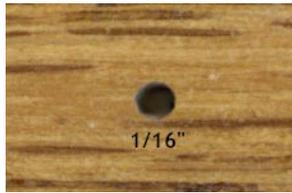
Figure 3. Lyctid powderpost beetle emergence hole in oak.
