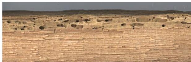
Figure 4. Anobiid powderpost beetle damage in softwood. Note that damage is absent in heartwood.
